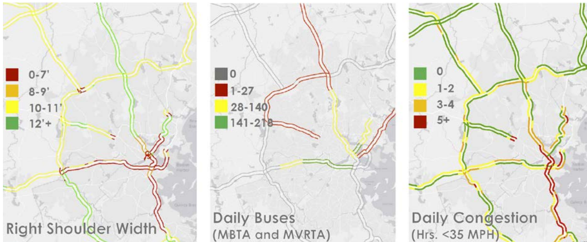
Figure 2.3: Corridor characteristics for bus-on-shoulder (Source: MassDOT, 2019a)
