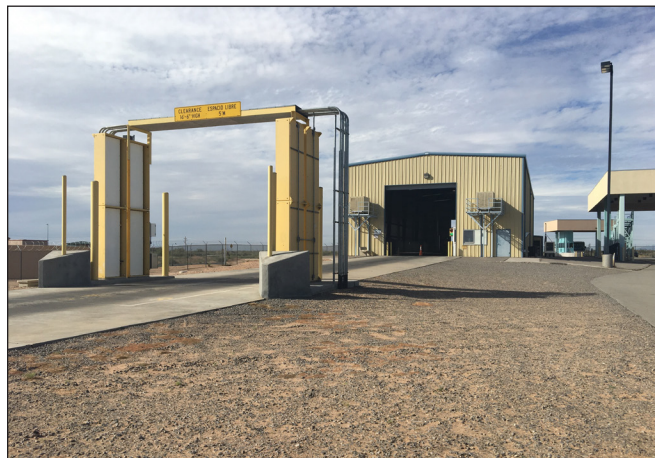
A freight x-ray scanner at the Santa-Teresa crossing in New Mexico. Source: J. Davis
