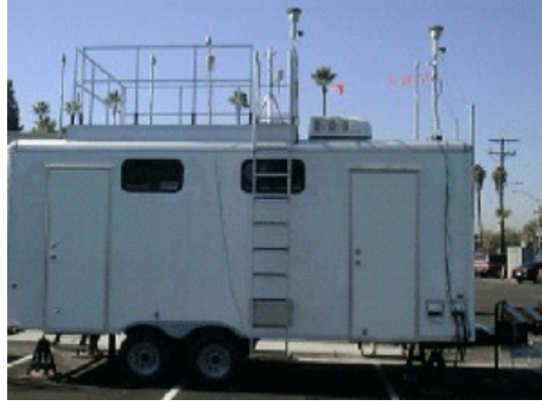
Figure 4. Mobile particle instrumentation unit from the UCLA-based Southern California Particle Center Supersite. Photo courtesy of the Southern California Particle Center Supersite.
