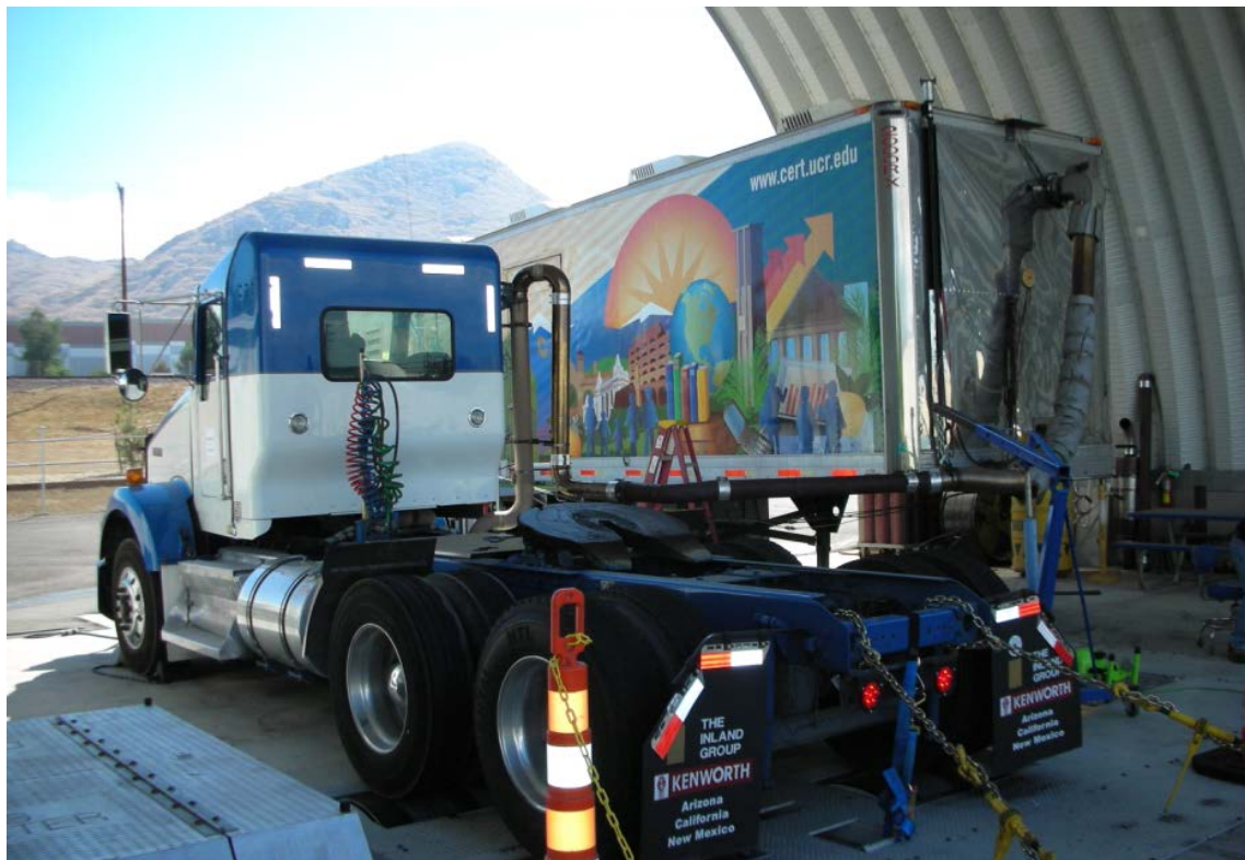
Figure 5-7. Truck being tested on the chassis dynamometer
