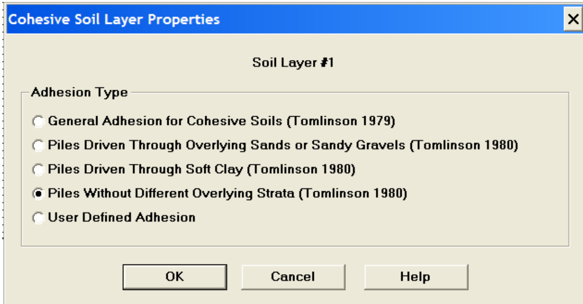
Figure 9-23. DRIVEN Cohesive Soil Layer Properties screen.
