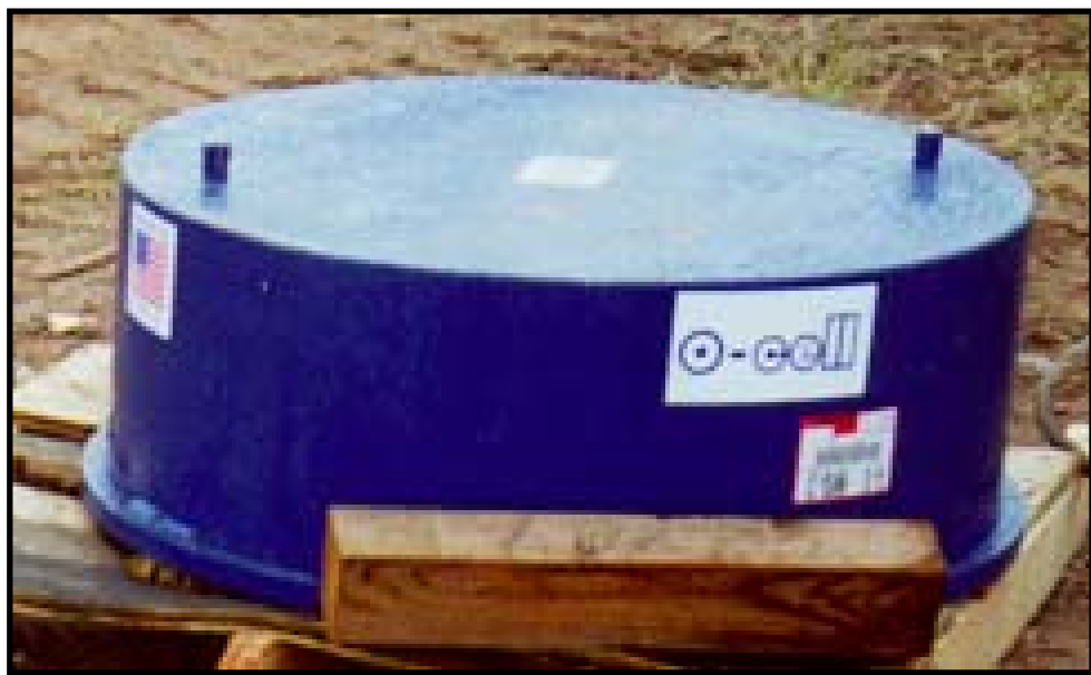
Figure 9-74. Photograph of an O-Cell ® .
