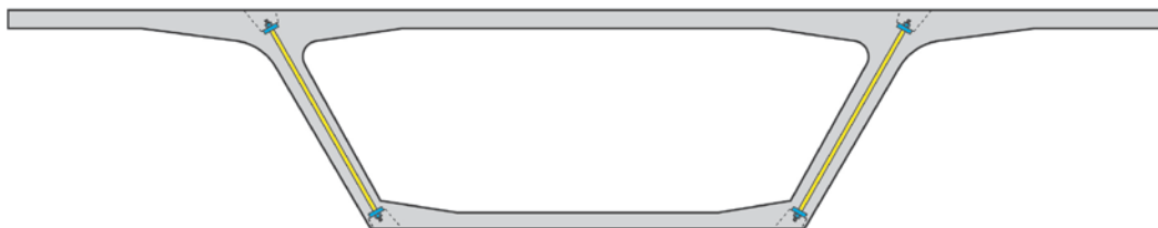
Figure 1.28 - Vertical Post-Tensioning in Webs
