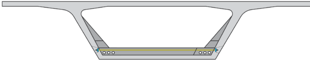
Figure 1.27 - Transverse Post-Tensioning in Deviator Ribs
