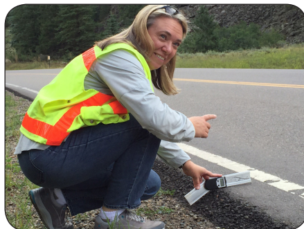
FLH Highway Safety Engineers collecting measurements of pavement edge slope and vehicle speed for project safety reviews.
