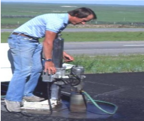
Exhibit 4-10 Proper Core Removal Device
