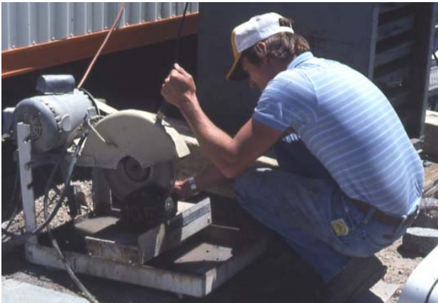
Exhibit 4-11 Sawing to Separate Pavement Layers
