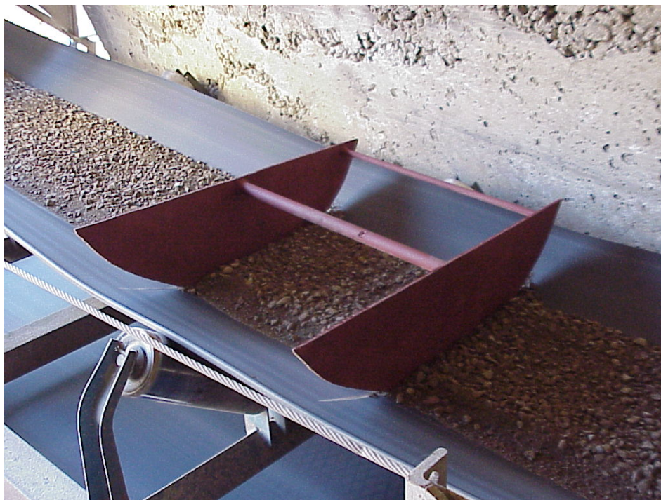
Exhibit 3-9 Proper Device for Belt Sampling
