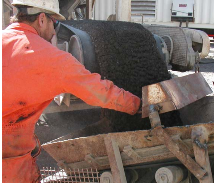
Exhibit 3-7 Sampling Device Cutting Across Flowing Stream
