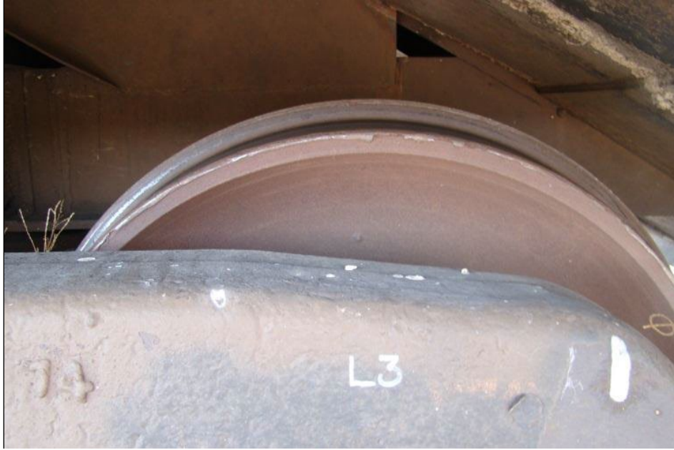
Figure 4. Wheel With Rolled Rim That Created Narrow Spikes in the Ultrasonic Data
