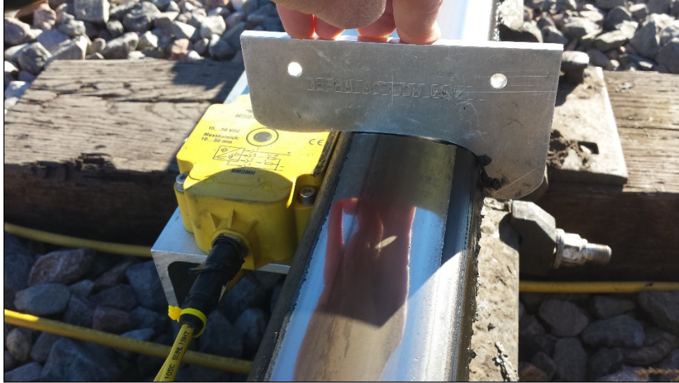
Figure 12. Clearance to Sensor with Worn Wheel Profile
