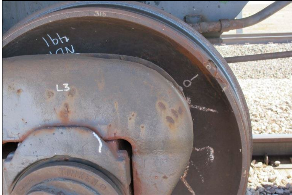
Figure 6. Shattered Rim that Caused the Indication in Figure 5
