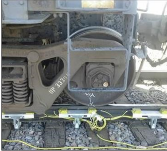
Figure 20. Test Wheel Notch Aligned on One of the Magnetic Sensors
