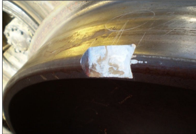
Figure 19. 0.75-inch Deep Rim Notch on the Test Wheel
