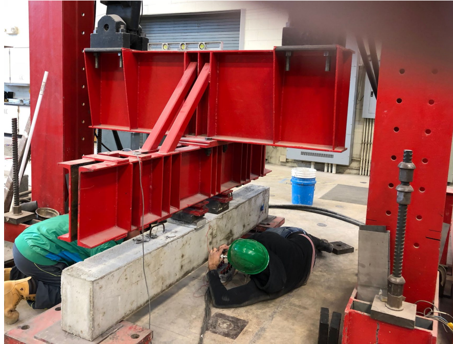
Figure 2-18 - Beams testing and crack monitoring
