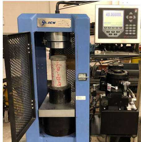
Figure 2-5 – Test setup for compressive strength
