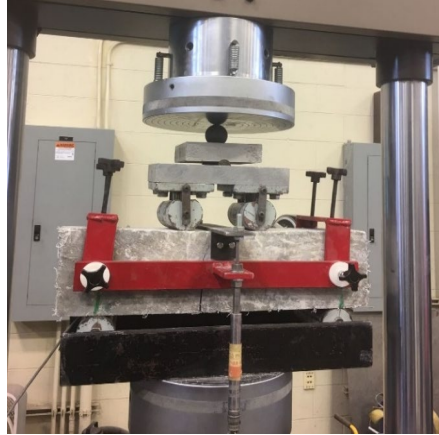
Figure 2-6 – Test setup for flexural strength measurement of beam specimens
