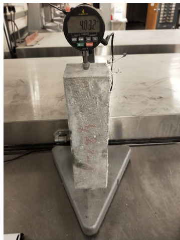
Figure 2-7 – Drying shrinkage measurement (a) drying shrinkage and (b) restrained expansion
