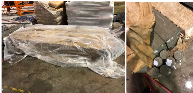
Figure 2-17 – Curing of beams and cylinders and occupying samples
