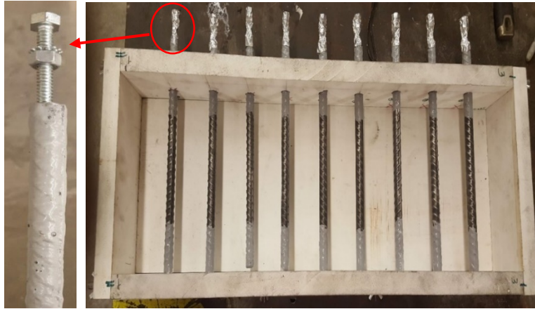
Figure 2-9 – Custom made corrosion test sample molds with epoxy-coated bars at ends
