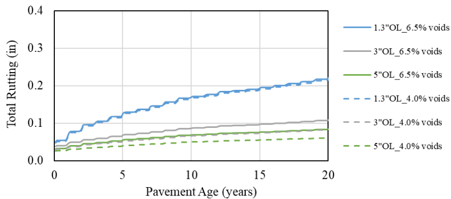
Figure 91. Impact of HMA air voids and overlay thickness on local calibration predicted total rutting for Missouri
