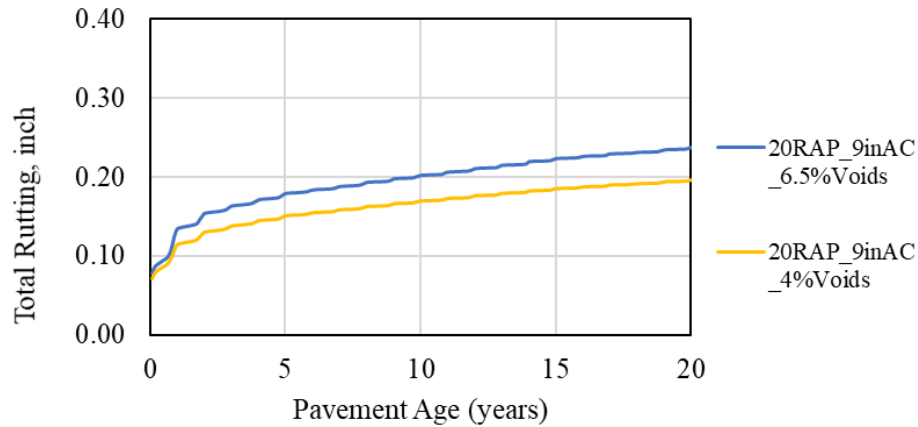
Figure 90. Impact of HMA air voids on local calibration predicted total rutting for Missouri
