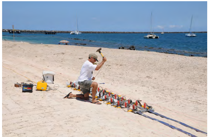
Figure 7. SR surveying with closely spaced geophone streamer
