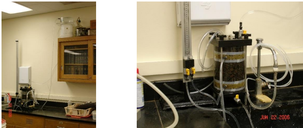
Figure 6-60. Layout of the Sand and Gravel Permeameter with the 3-Fine material inside.
