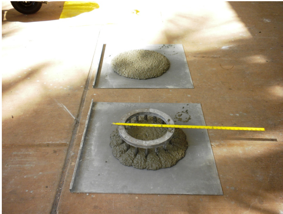
Figure 2: Typical slump flow and J-ring tests
