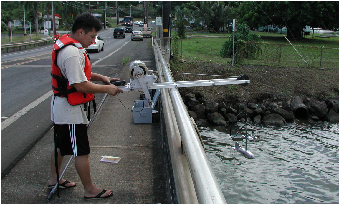
Figure 4-10: Sounding reel and Price meter at Kahaluu Bridge
