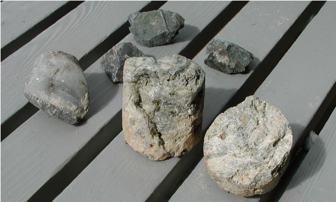
Figure 3-18: Boring samples (hard coral rocks) at 7-10 ft depth at Kaelepulu Bridge
