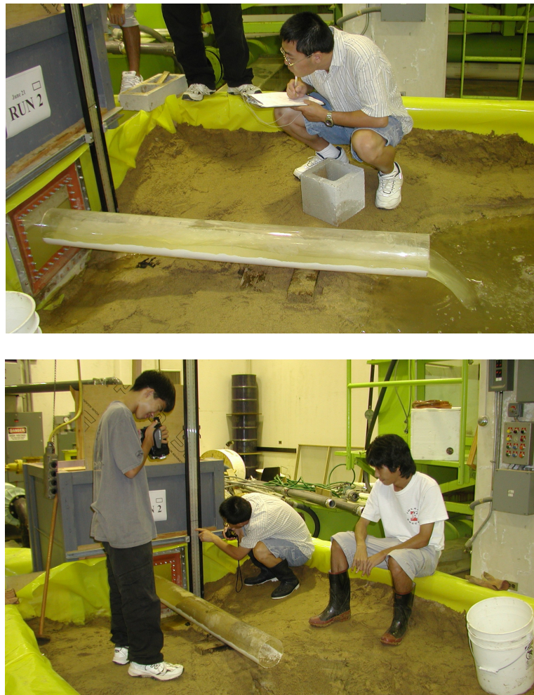
Figure 8-6: Photographs of model circular culvert experiment for Punaluu culvert
