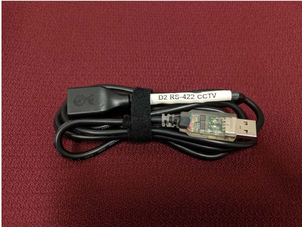
Figure 5.10: HHDC kit USB serial RS-422 to D2 CCTV RJ45 connector
