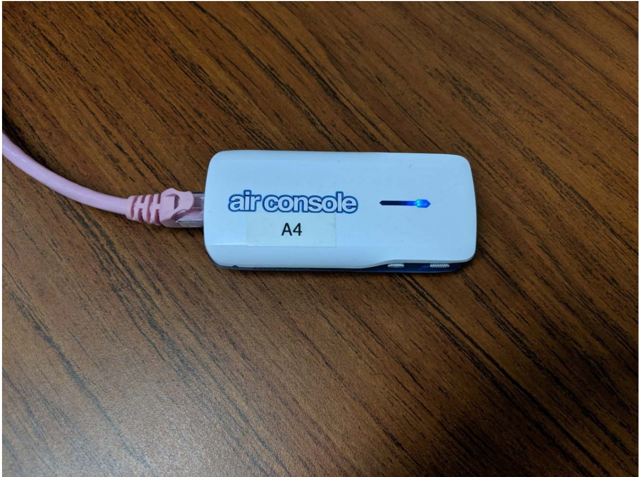
Figure 5.7: HHDC Airconsole connected to Ethernet
