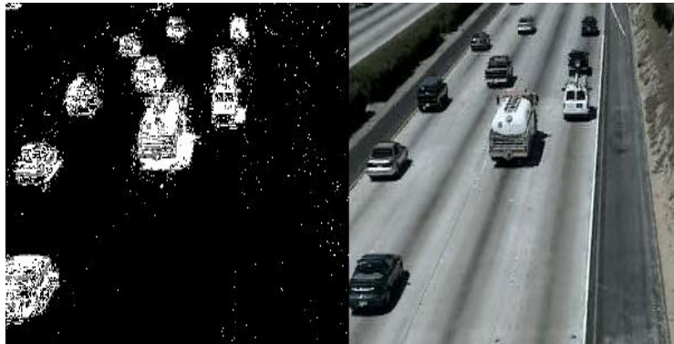
Figure 4. Background subtraction using Gaussian Mixture Model
