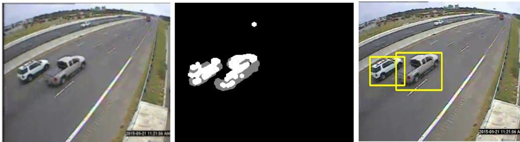
Figure 5. Background subtraction and contouring
