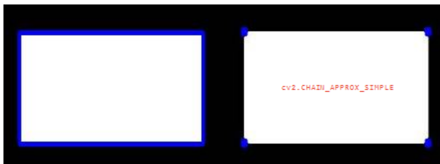
Figure 6. OpenCV Contour approximation method
