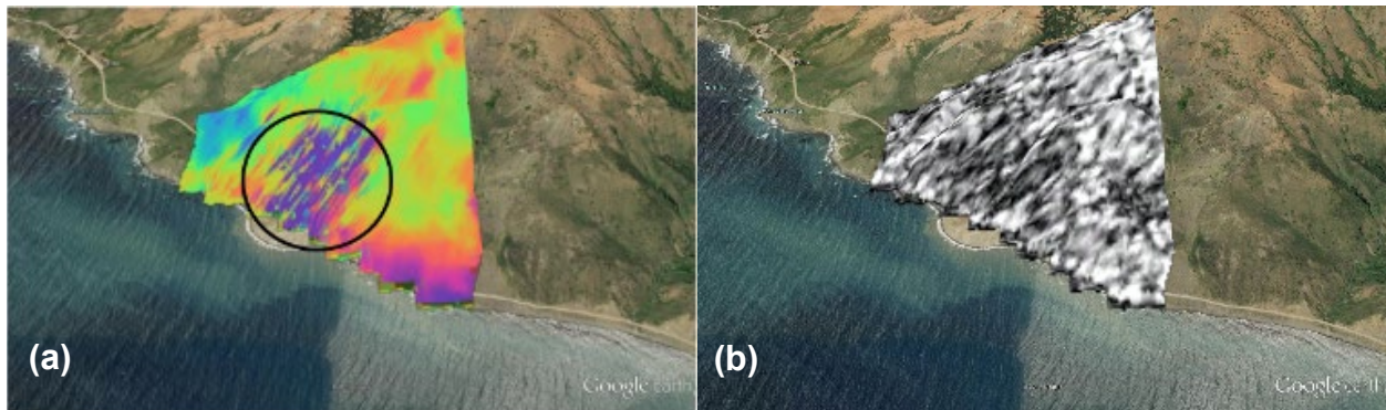
Figure 44: Test 1: (a) Phase map shows disturbances in the area where landslide occurred; (b) Coherence map
