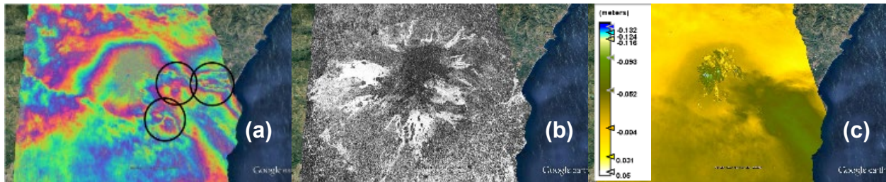
Figure 42: Test 3: (a) Phase map shows slope instability and possible landslide activity; (b) Coherence map shows low signal strength inside the crater as in the other tests; (c) Displacement map showing a displacement activity in the order of 10 cm
