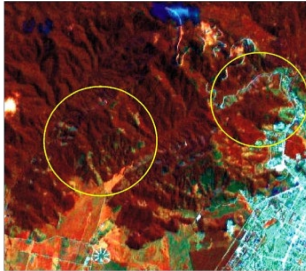
Figure 6: In this image landslides were detected using IHS image fusion technique. (Marcellino, et al., 2009)
