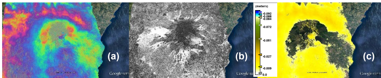
Figure 41: Test 2: (a) Phase map shows no significant variations that signify slope instability; (b) Coherence map shows low signal strength near the crater; (c) Displacement map showing a minor subsidence around the crater
