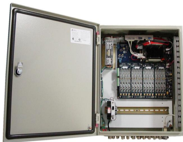
Figure 4.1: Sensor Highway II – data acquisition system
