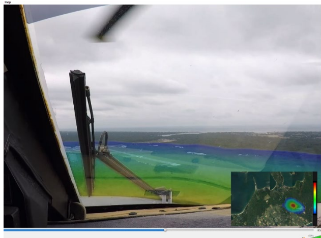
Figure 47. Example screenshot of cockpit noise overlay video. This video depicts an S-76 approach to KHTO.
