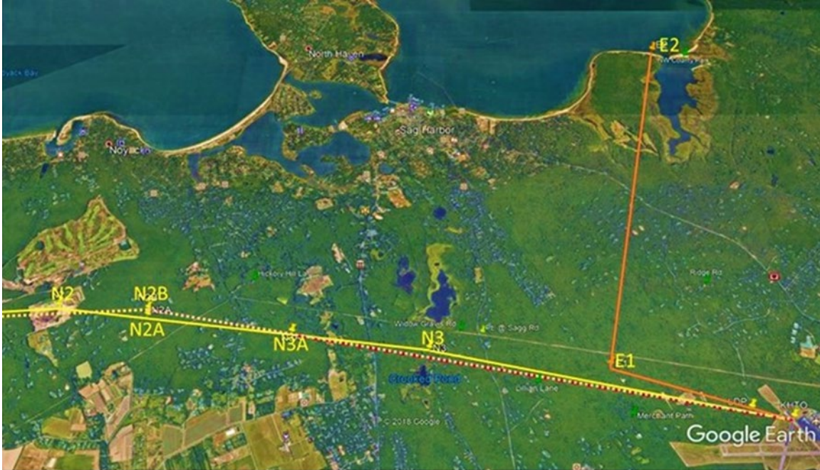
Figure 4. Flight Tracks for Current (Nov 0, solid line) and Proposed (dotted lines) KHTO November Noise Abatement Arrival Procedures
