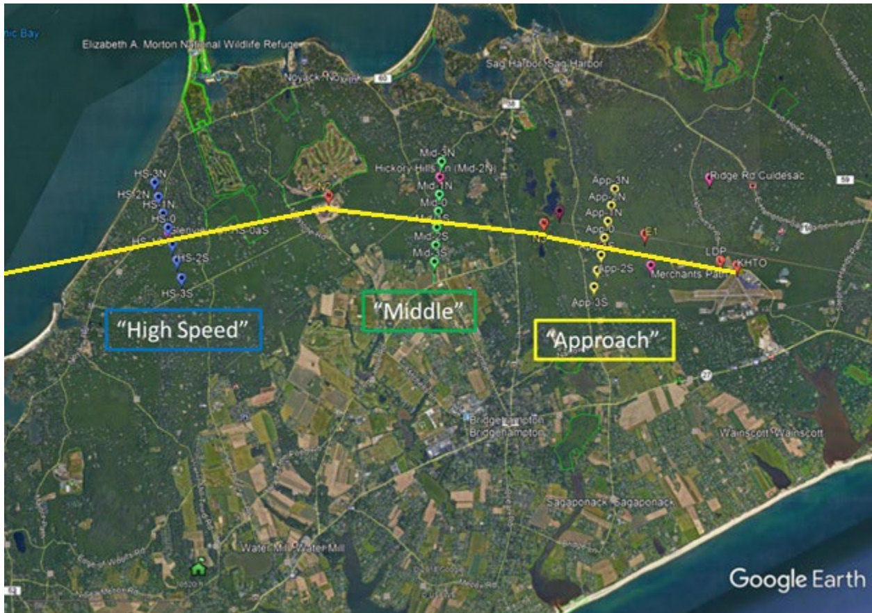
Figure 5. AAM Analysis locations (lateral points) 1000, 2000 and 3000 ft to the North (N) and South (S) of the ground track during ‘high speed’, ‘middle’ and ‘approach’ segments of November Noise Abatement Arrival Route
