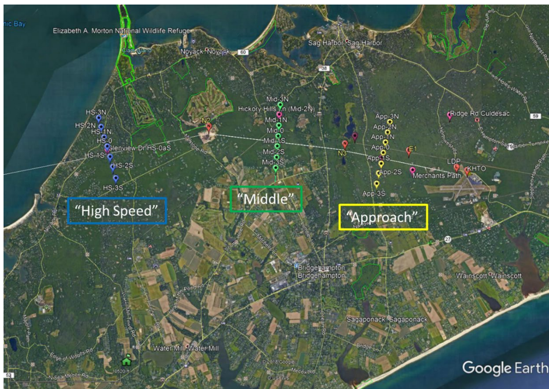
Figure 48. AAM Analysis locations (lateral points) 1000, 2000 and 3000 ft to the North (N) and South (S) of the flight track during 'high speed', 'middle' and 'approach' segments of November Noise Abatement Arrival Route
