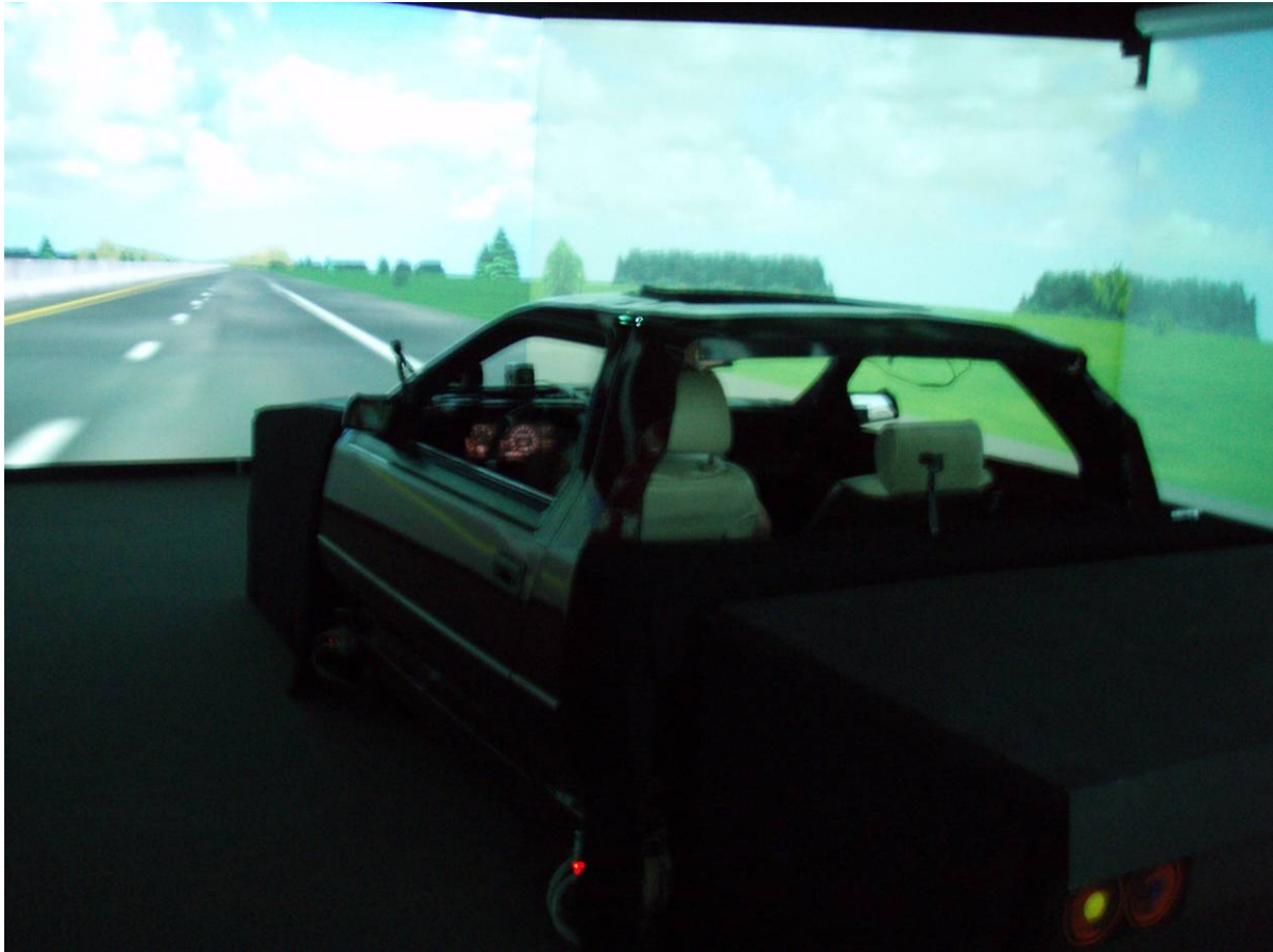
Figure 7. Simulator cab, front screen, front-right screen, and front-side screen
