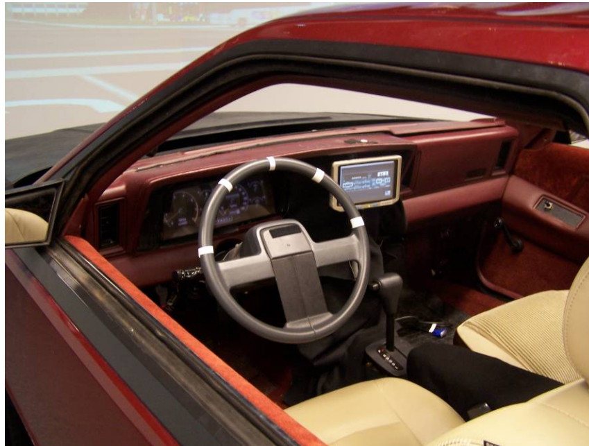
Figure 9. View of the inside of the simulator cab Note: The instrument panel configuration is from a prior study.
