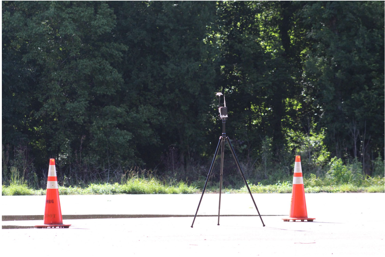
Figure 5.6: RTK ground station.
