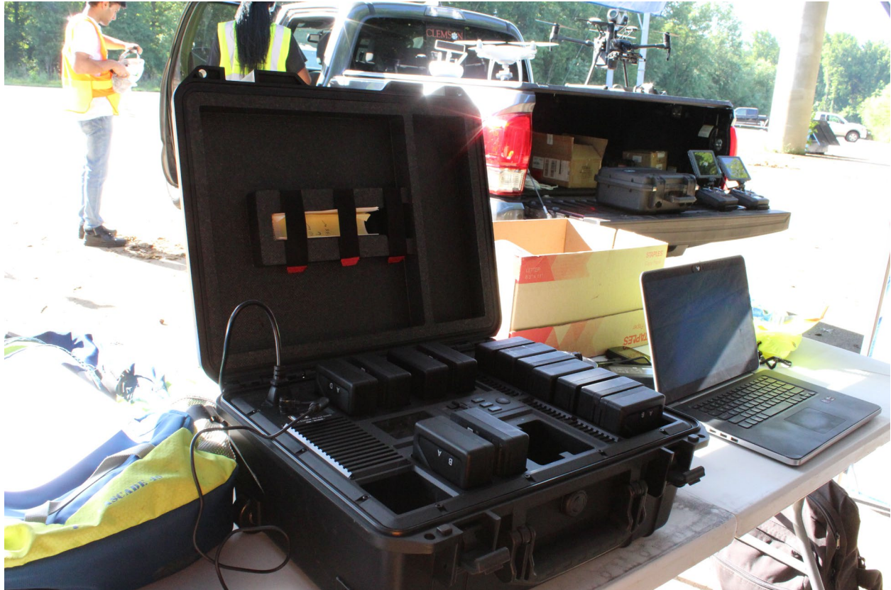
Figure 5.7: TB50 battery charging hub.
