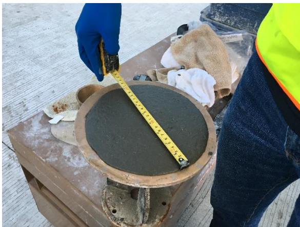
Figure C3: UHPC Flow Test
