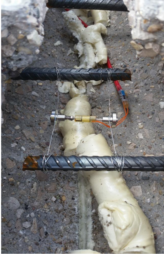
Figure B9: Transverse Shear Key Gage
