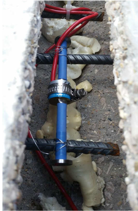
Figure B10: Longitudinal Shear Key Gage
