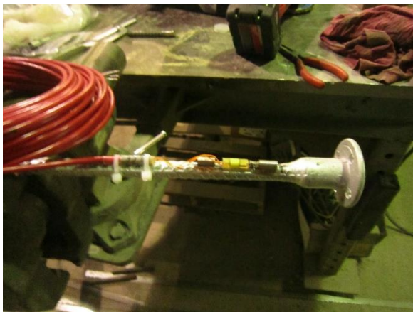
Figure B6: Instrumented Dowel Bar
