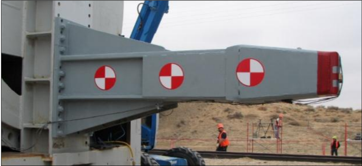
Figure 9. Ram Arm with 12-inch by 12-inch Indenter
