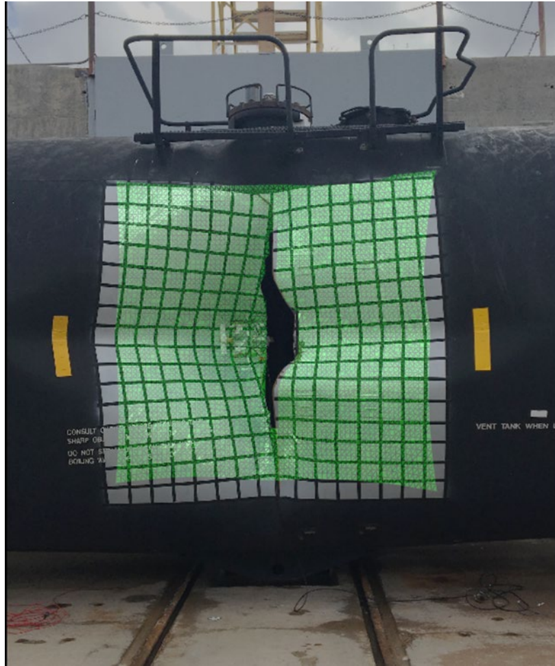
Figure 24. Composite Image of Scan Geometry Overlaid on Photograph of Post-test Tank Car
