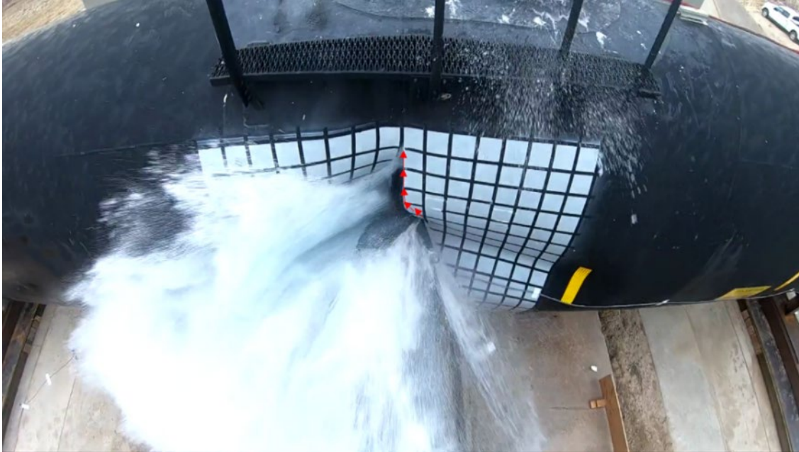
Figure 20. Third Frame Extracted from Onboard Ram Car Video Showing Direction of Tear Propagation at Extent of Tearing
