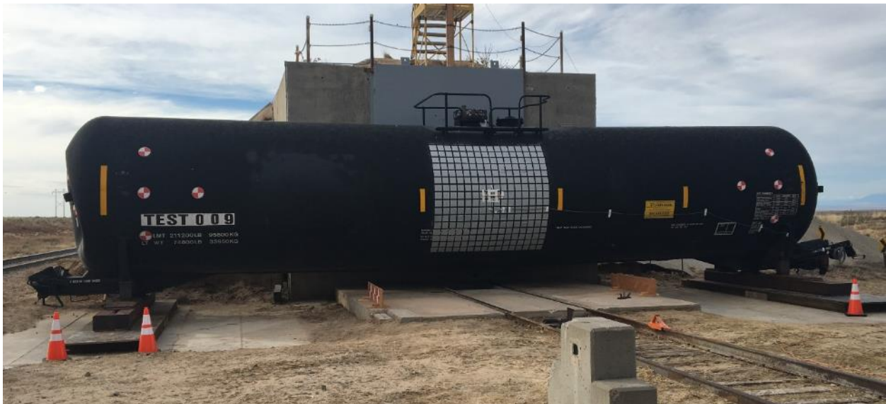
Figure 5. Target Tank Mounted on Support Skids
