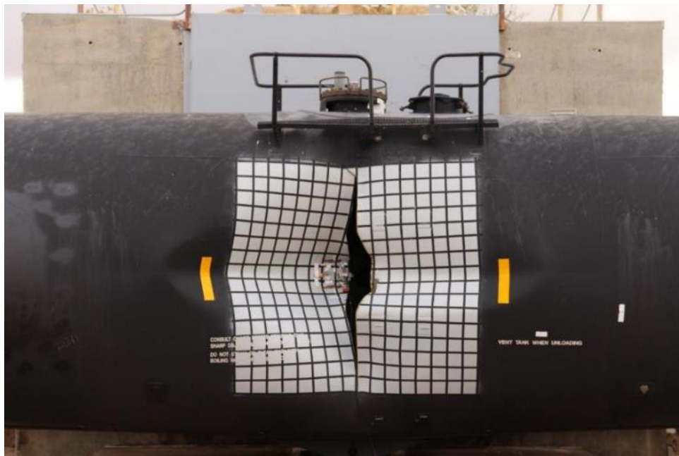
Figure 16. Tank Car after the Impact (impact side)
