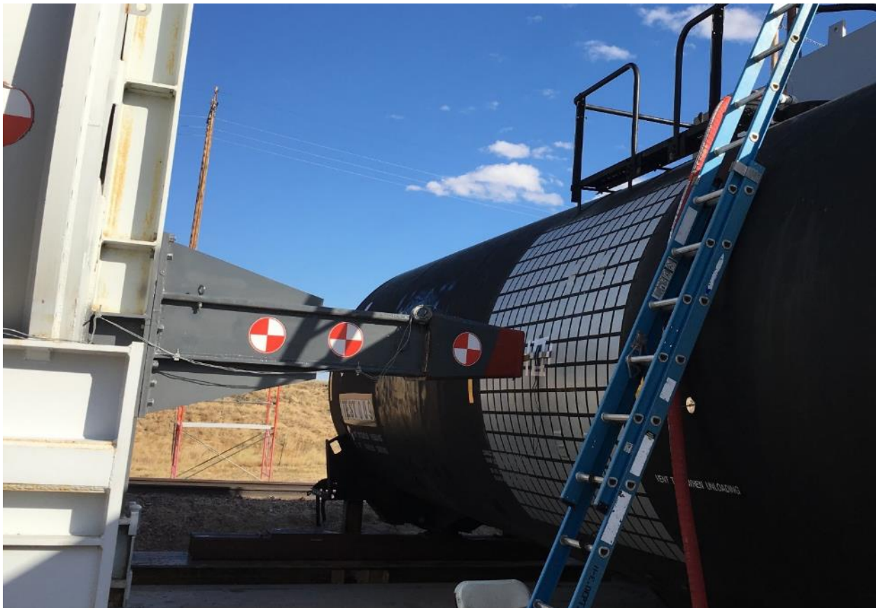
Figure 10. Ram Arm with 12-inch by 12-inch Indenter Aligned with Center of the Tank Car
