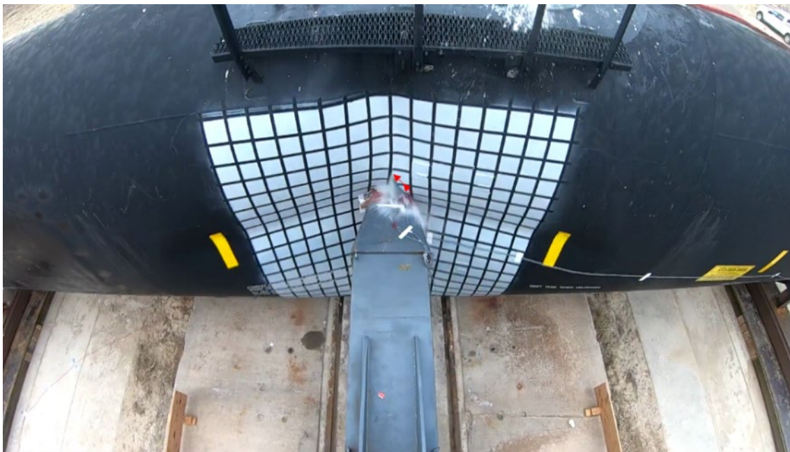
Figure 19. Subsequent Frame Extracted from Onboard Ram Car Video Showing Direction of Tear Propagation
