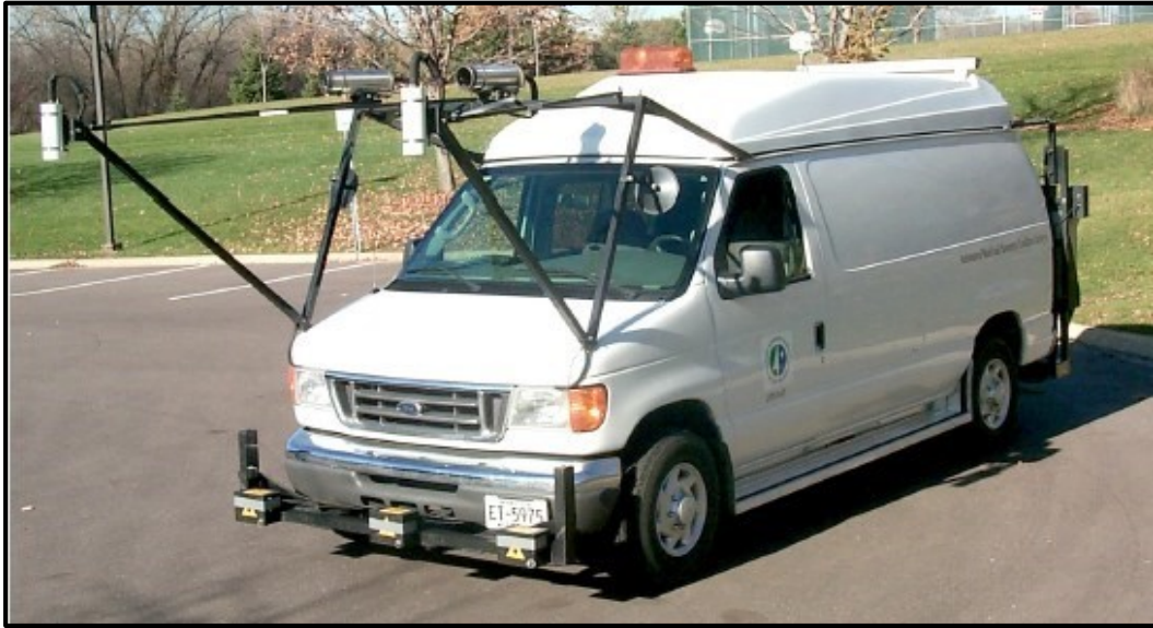
Figure 7: MnDOT’s Pathway Services, Inc. Digital Inspection Vehicle (DIV) [from Janisch (2006)]
