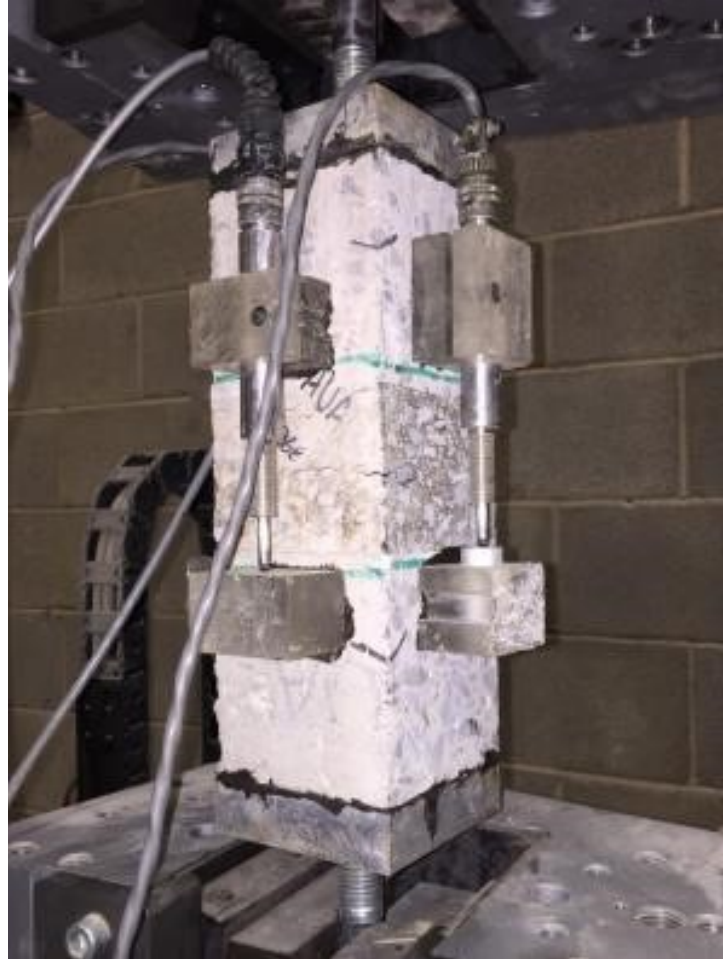
Figure 32: Schematic of direct tension test; at right, laboratory direct tension test on specimen with HMA interlayer
