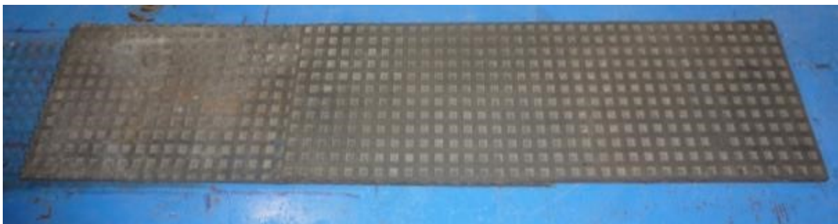
Figure 22: Neoprene pads used to simulate support conditions
