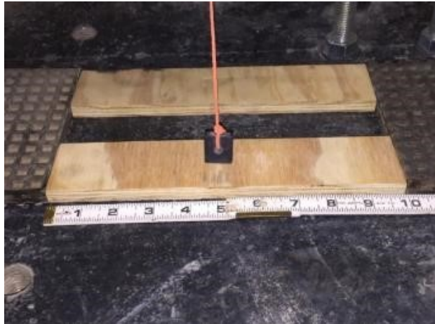
Figure 31: 10-inch Gap in Fabcel with Plumb Bob to Center the Gap
