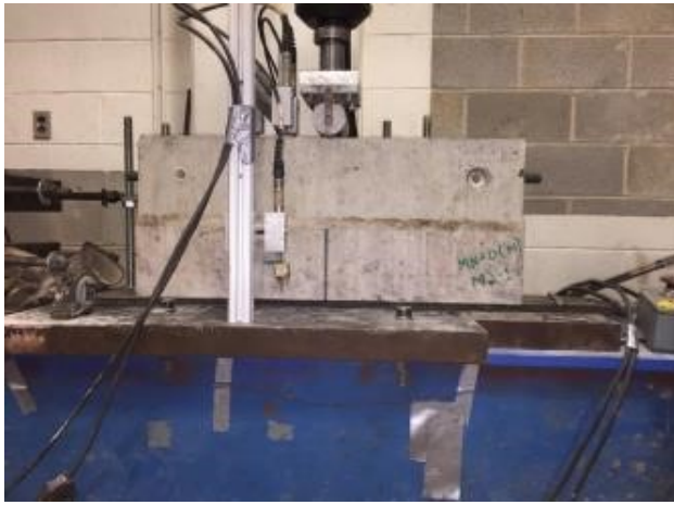
Figure 30: Final test apparatus for reflective cracking
