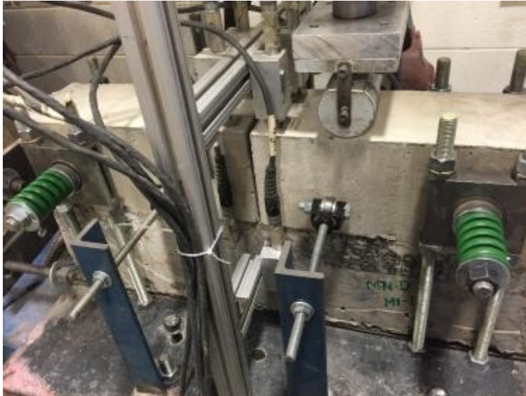
Figure 21: Test setup used to characterize deflection at the interface
