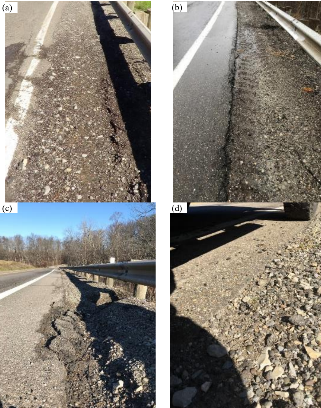
Figure B.8 Pictures from section one evaluation after: a. One month b. Four months b. Four months (Failed section) c. One year
