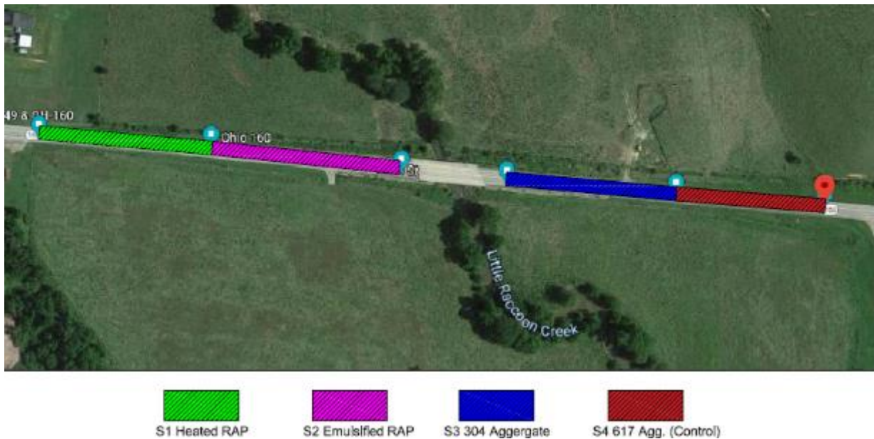
Figure A.3 Layout of test section on SR 160 in ODOT Vinton County
