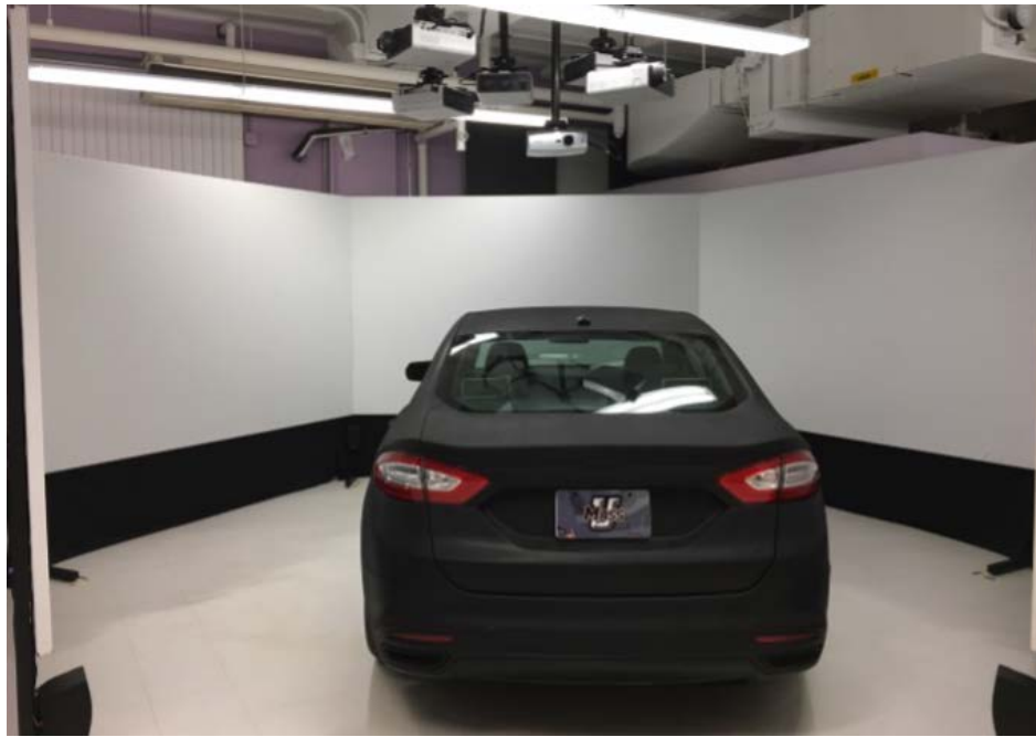
Figure 3.1 – Full-immersion driving simulator
