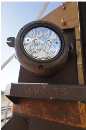
Hydra-Tech single auxiliary light on locomotive
