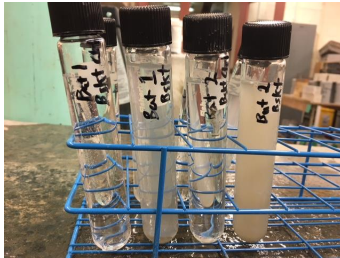
Figure 8. Solutions Obtained After Submerging the Concrete in a Basket as Specified in the USACE Test Procedure. USACE = U.S. Army Corps of Engineers.
