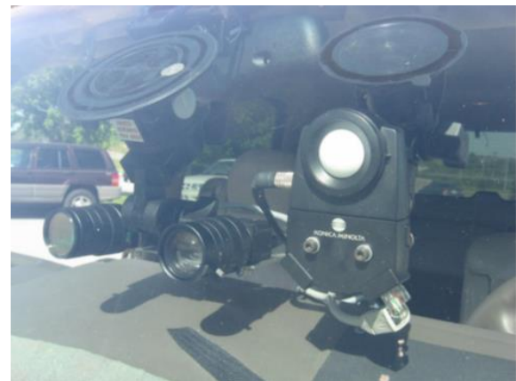
Front Windshield RLMMS Equipment (Color and Luminance Cameras left, Illuminance Meter right)
