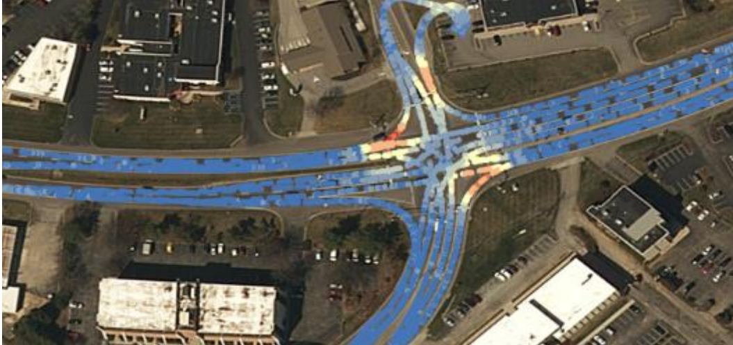
Figure 6. Examples of Intersection Lighting Measurement Points. Measurements are color-coded based on horizontal illuminance values, with red indicating higher illuminance and blue indicating lower illuminance.
