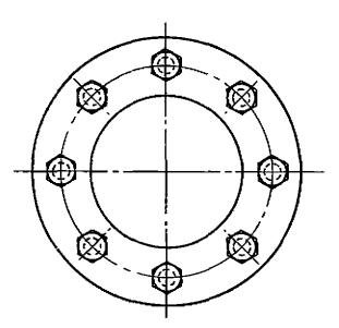
FIGURE 1. Permeability cup assembly
