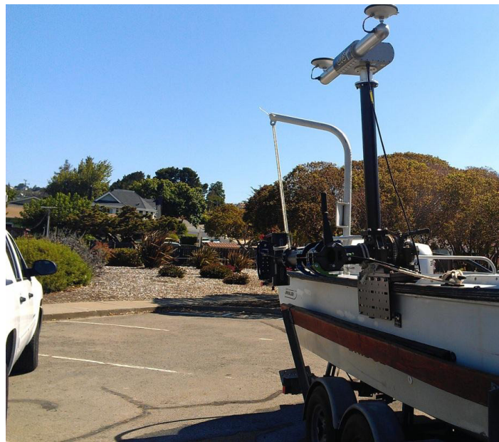
Figure 21. Photo. 3D real-time multibeam sonar mounted on the boat.
