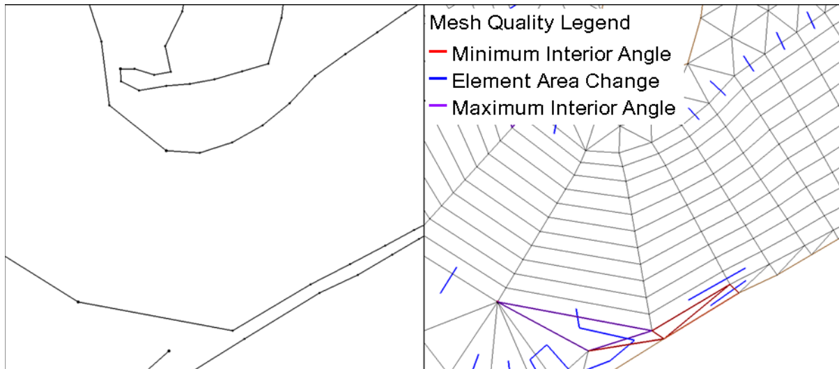
Figure 5.18. Element quality concerns in transition regions.
