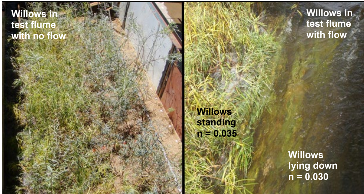
Figure 4.30. Calibrated n values for willows standing and lying down in flowing water.
