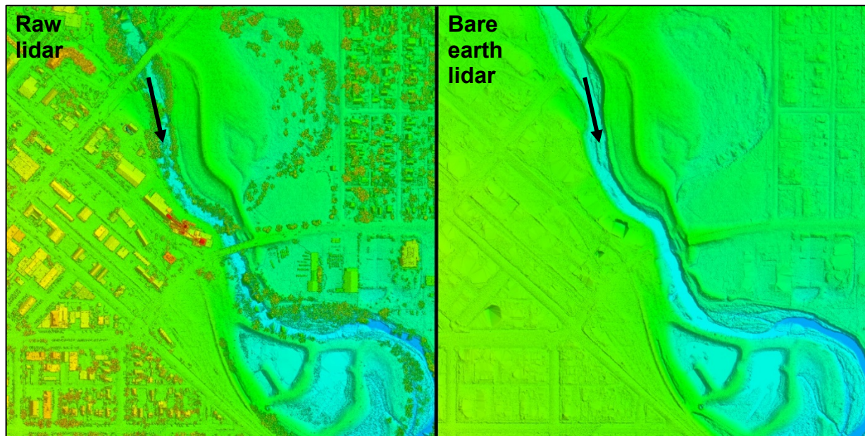
Figure 4.11. Raw vs. bare earth triangulated lidar data.
