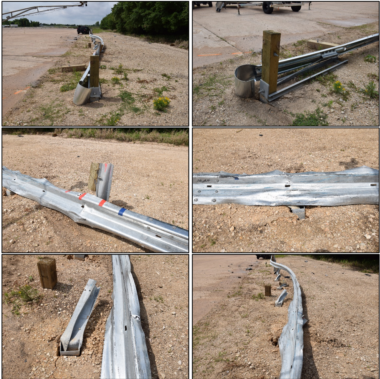
Figure 7.3. Terminal after Test No. 611011-1.
