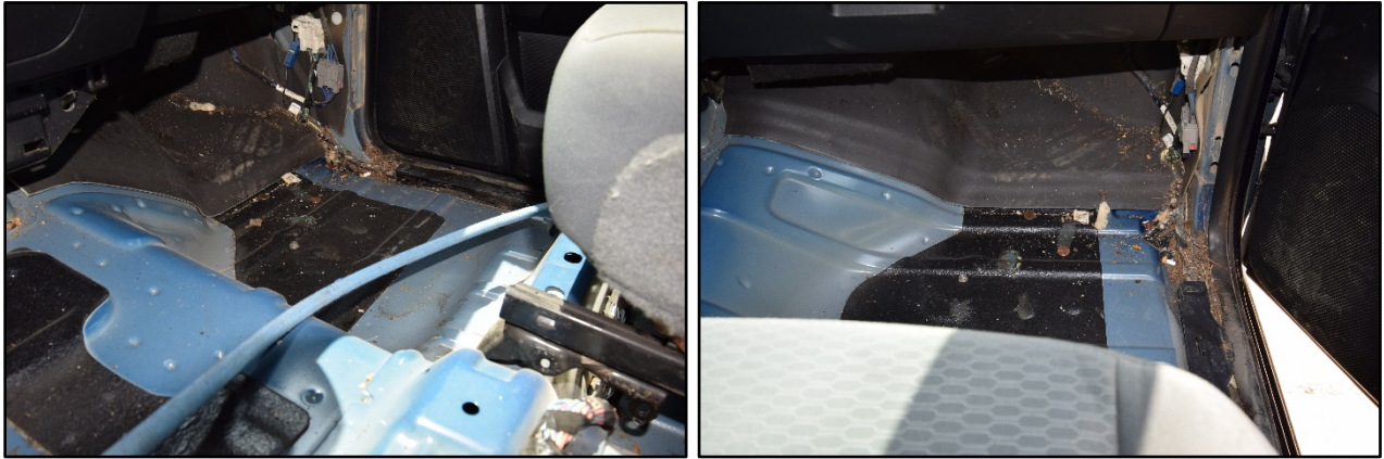
Figure 7.6. Front Impact-Side Interior of Test Vehicle after Test No. 611011-1.
