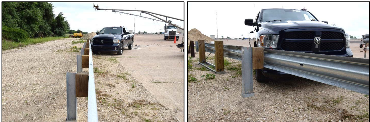
Figure 7.1. Terminal/Test Vehicle Geometrics for Test No. 611011-1.
