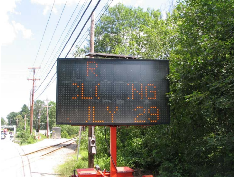
Figure 17. Photo. Variable message sign alerting travelers of upcoming roadway closure.
