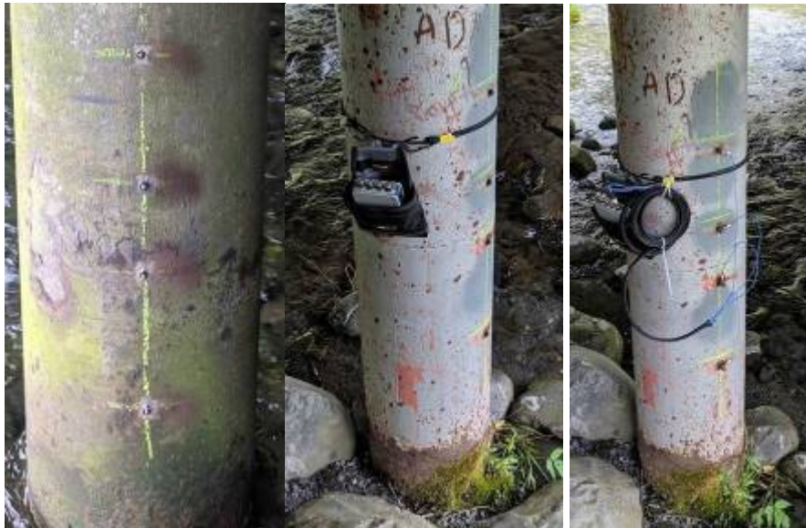
Figure 4: (a) Stud mounts for sensors (b) Sensor and DAQ Mounting (c) Connecting equipment
