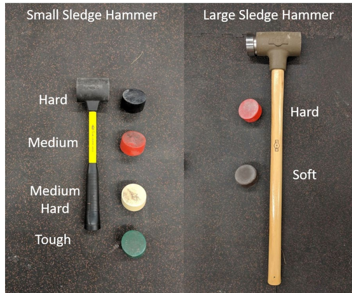
Figure 8: Different hammers and tips used for testing
