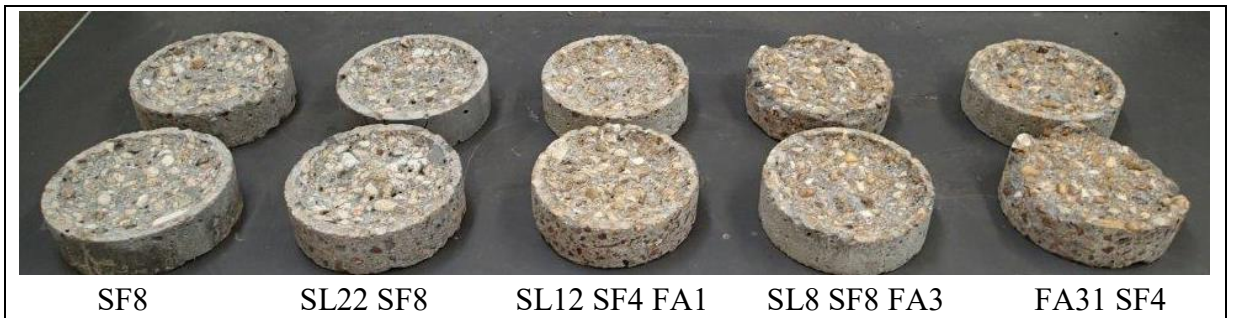
Prall samples after testing (Bowthorpe, 2019)
