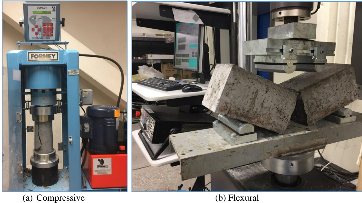
Figure 3.5 Compressive and flexural strength testing
