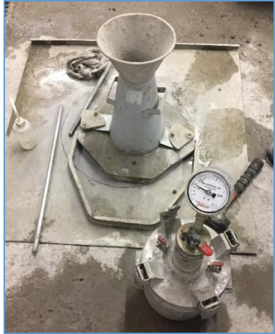
(a) Slump and air meter equipment
