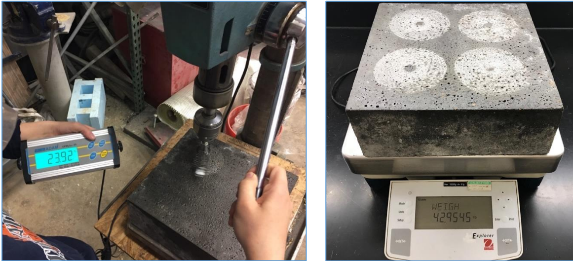
(a) Applying force to sample (b) Measuring mass loss
