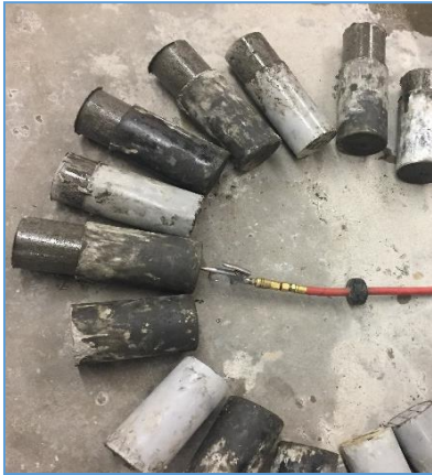
(c) Unmolding cylinders
