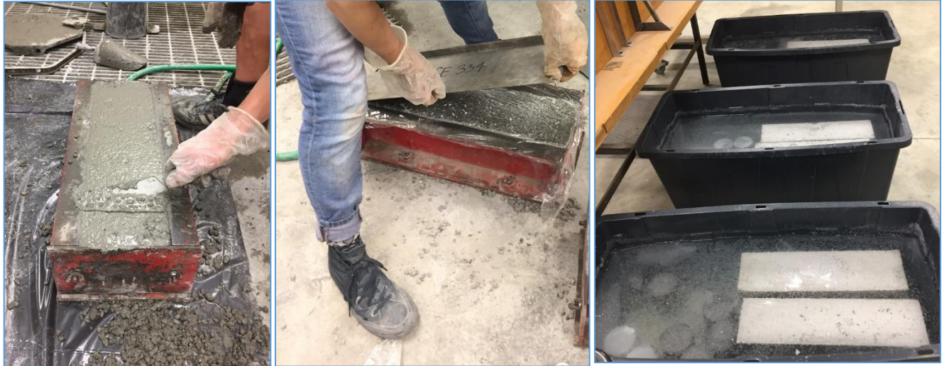
(a) Finishing samples (b) Covering samples (c) Samples curing
