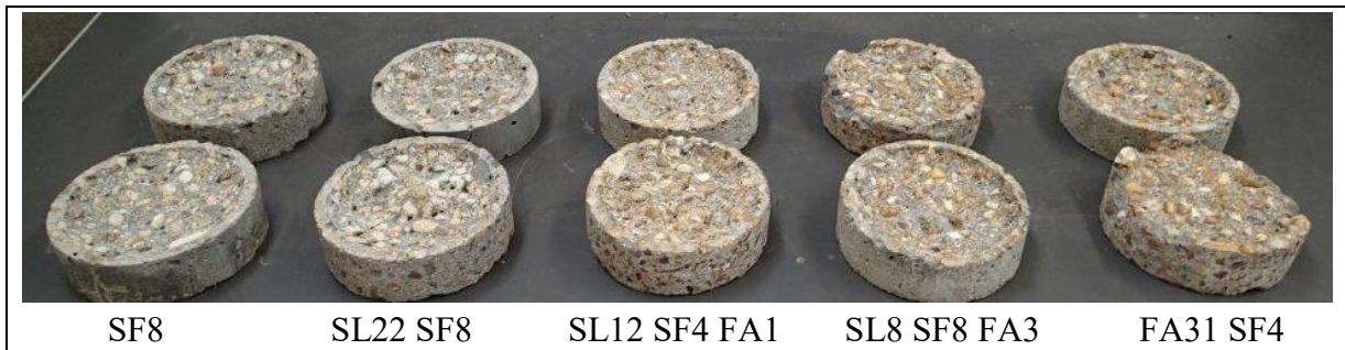
Figure 4.13 Prall samples after testing (Bowthorpe, 2019)
