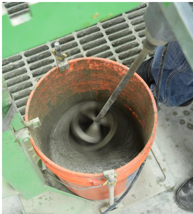
Figure 1-3. Paddle mixing of grout
