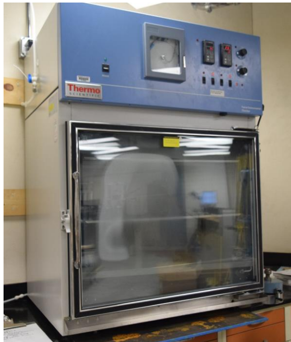
Figure 1-1. Moisture cabinet at the UAF laboratory
