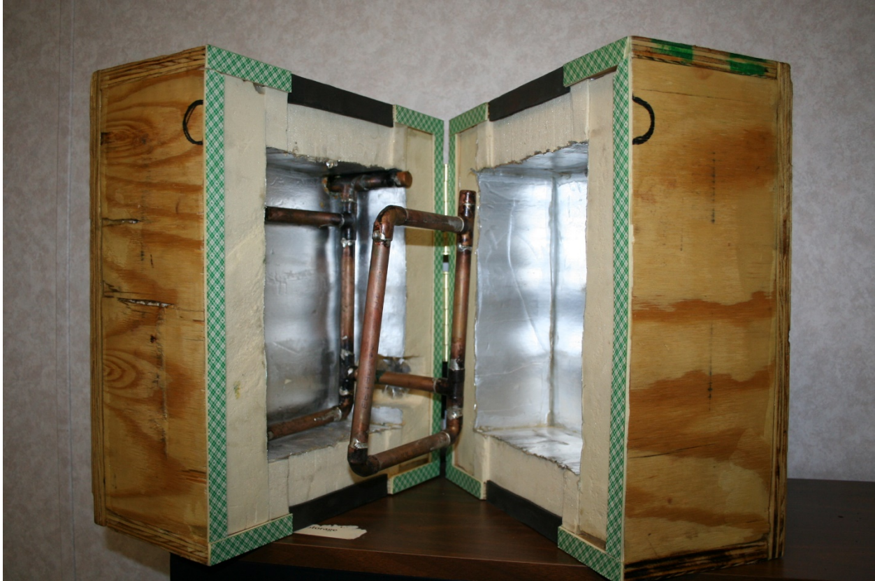
Figure 63. Photo. Temperature chamber.
