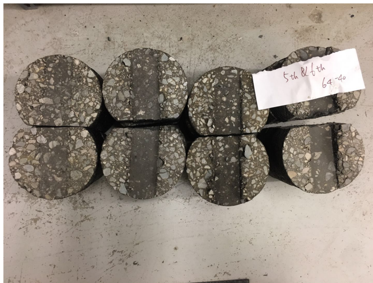
Figure 3.11 HWT specimens after testing
