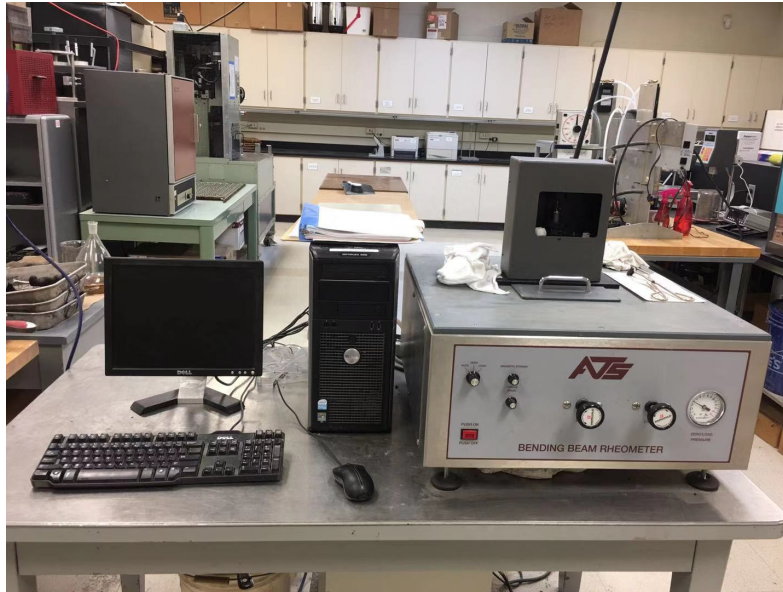
Figure 3.5 the BBR equipment
