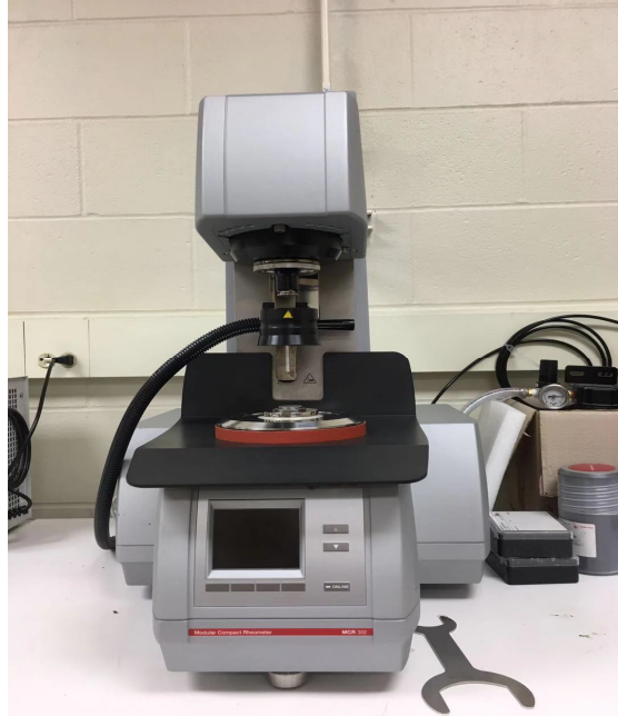
Figure 3.4 the DSR equipment
