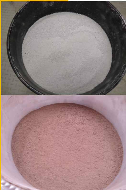
Images represent two of the 11 pozzolanic materials. The material in the black container (top) is the natural pozzolan, and the material in the white container (bottom) is the fluidized bed combustion fly ash. © Purdue University, Lyles School of Civil Engineering.
