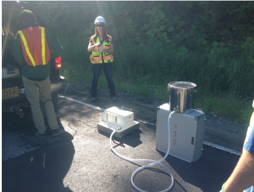
Photo 4: Dynamic Friction Tester with Case and Water Source
