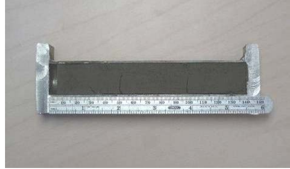
Figure 34. Photo. Bar linear shrinkage test.
