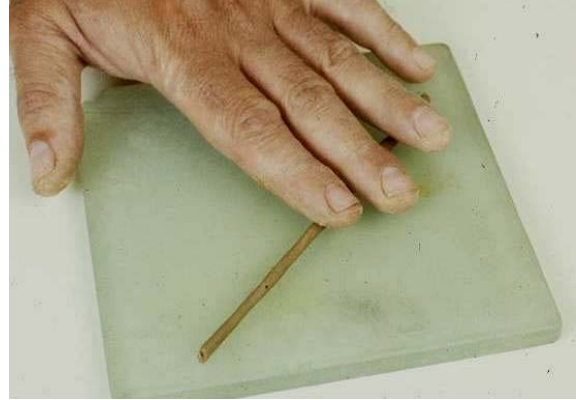
Figure 31. Photo. Plasticity test.
