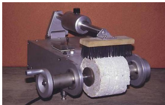
Figure 55. Photo. Abrasion resistance test.
