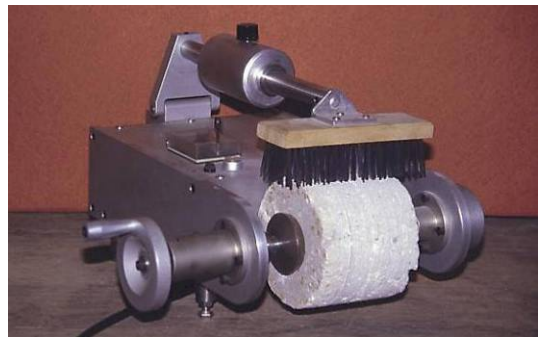
Figure 55. Photo. Abrasion resistance test.
