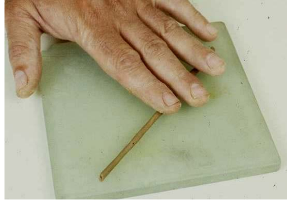
Figure 31. Photo. Plasticity test.
