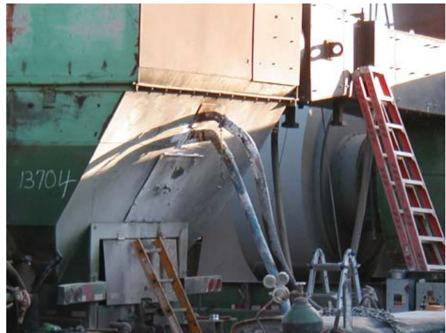
Figure 6 ~ Injection ports at the end of the drum: top port — asphalt binder, bottom port — warm mix additive.
