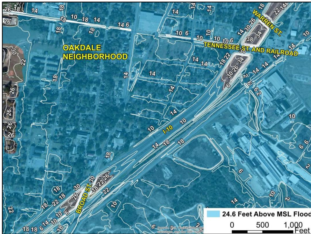
Figure 81: Hurricane Katrina Shifted + Intensified+ SLR Flood Zone in the Vicinity of the I-10 Study Segment, Flood Elevation 25 Feet (7.6 Meters)
