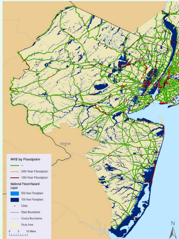
Figure C.14. Map. Potential exposure of the National highway system in New Jersey to inland flooding.
