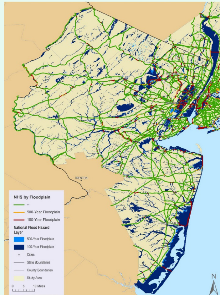
Figure 4.15. Map. Potential exposure of the National highway system in New Jersey to inland flooding.
