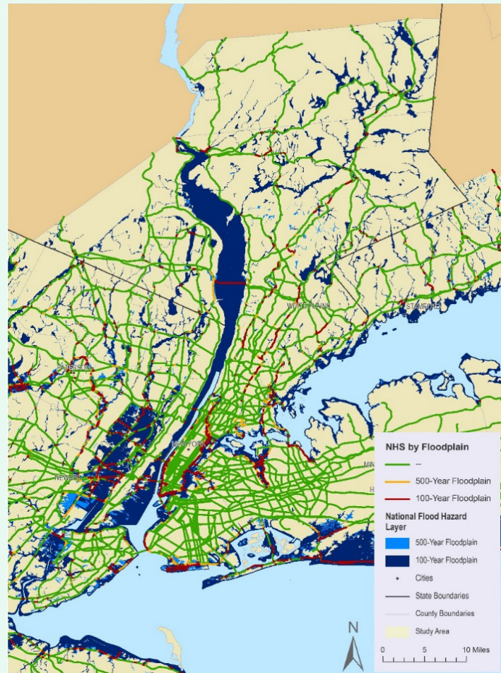
Figure 4.10. Map. Potential exposure of the National highway system in New York City and lower Hudson Valley to inland flooding.
