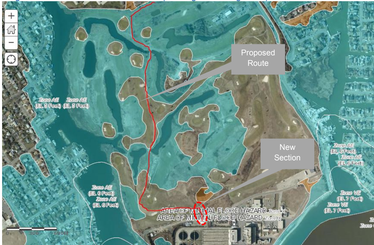
Figure 3: Recommended Route through the Bergen Point Golf Course from Kirby Lane to the Bergen Point Wastewater Treatment Plant (Utilizing an Existing Route)
