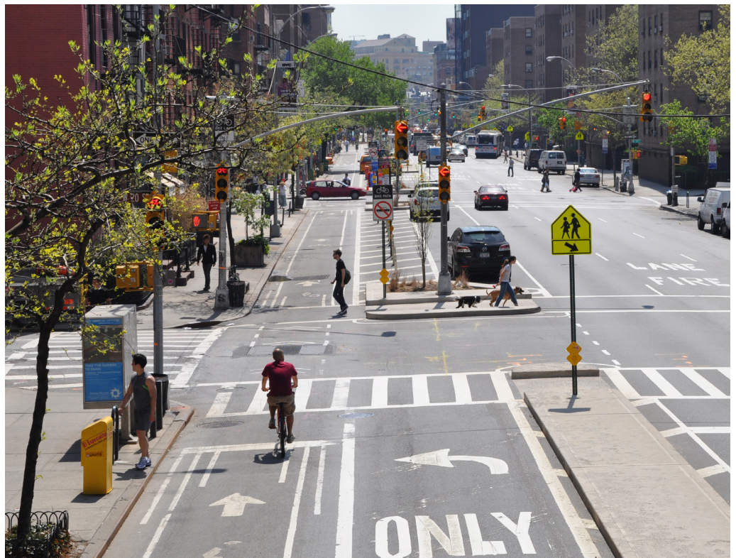
Dedicated bicycle signalization along New York City's 9th Avenue separated bike lane. (Source: NYC DOT)
