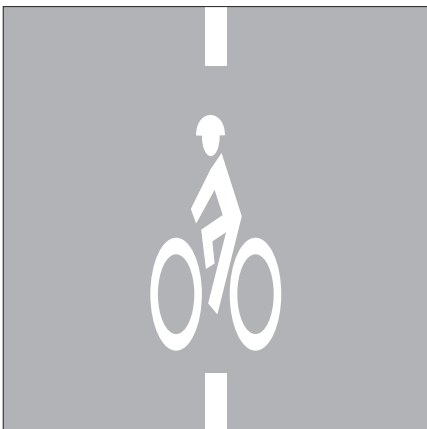
Bike detector pavement marking MUTCD Fig. 9C-7
