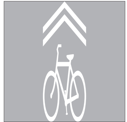
Shared lane marking MUTCD Fig. 9C-9
