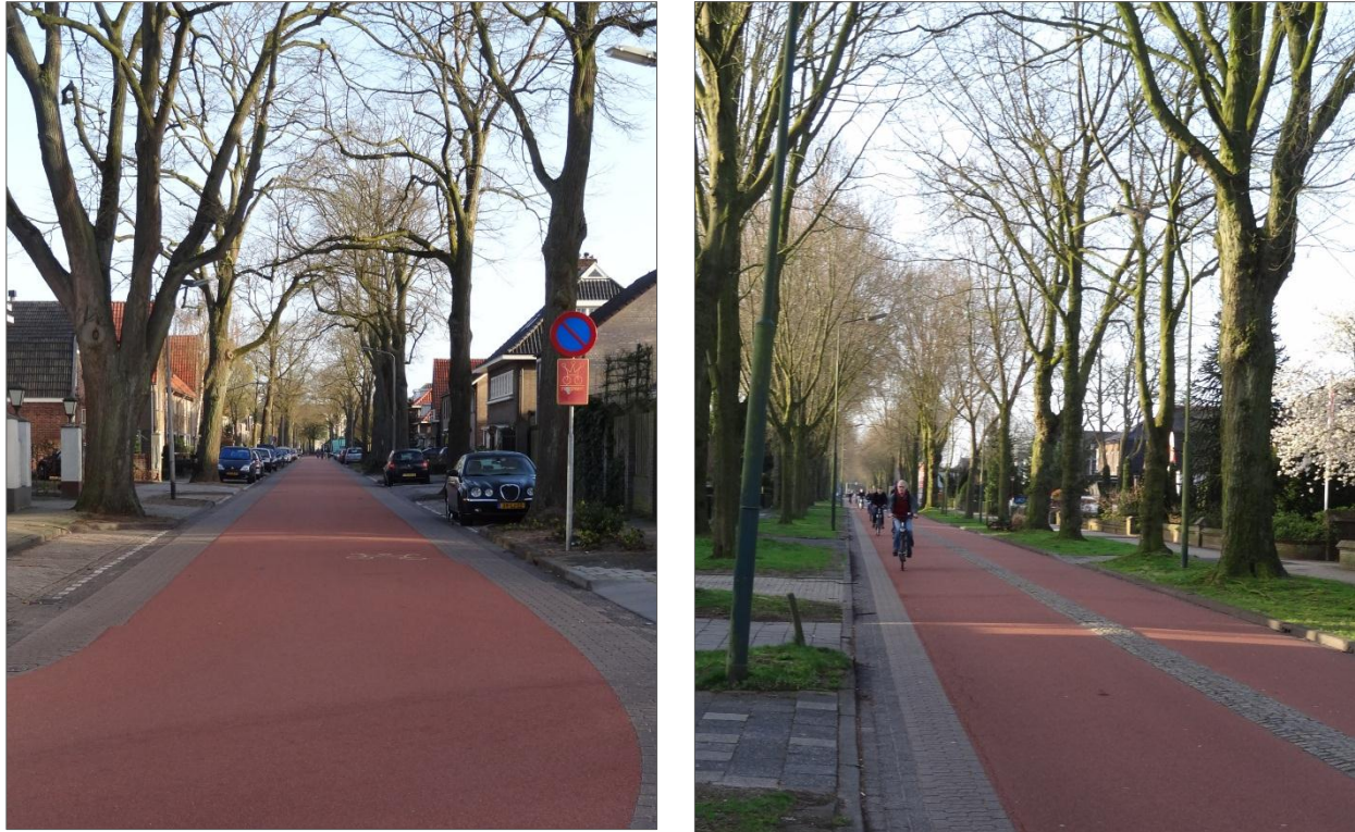
Figure 11. One lane, with on-street parking, and two-lane priority bicycle streets in Oss, the Netherlands.
