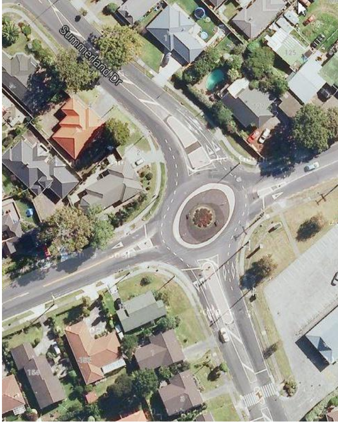
Figure 4. Example of Wider Median Island, Larger Raised Circle, Narrow Approach Lanes, and Circulating Lanes of Cyclist-Roundabout
