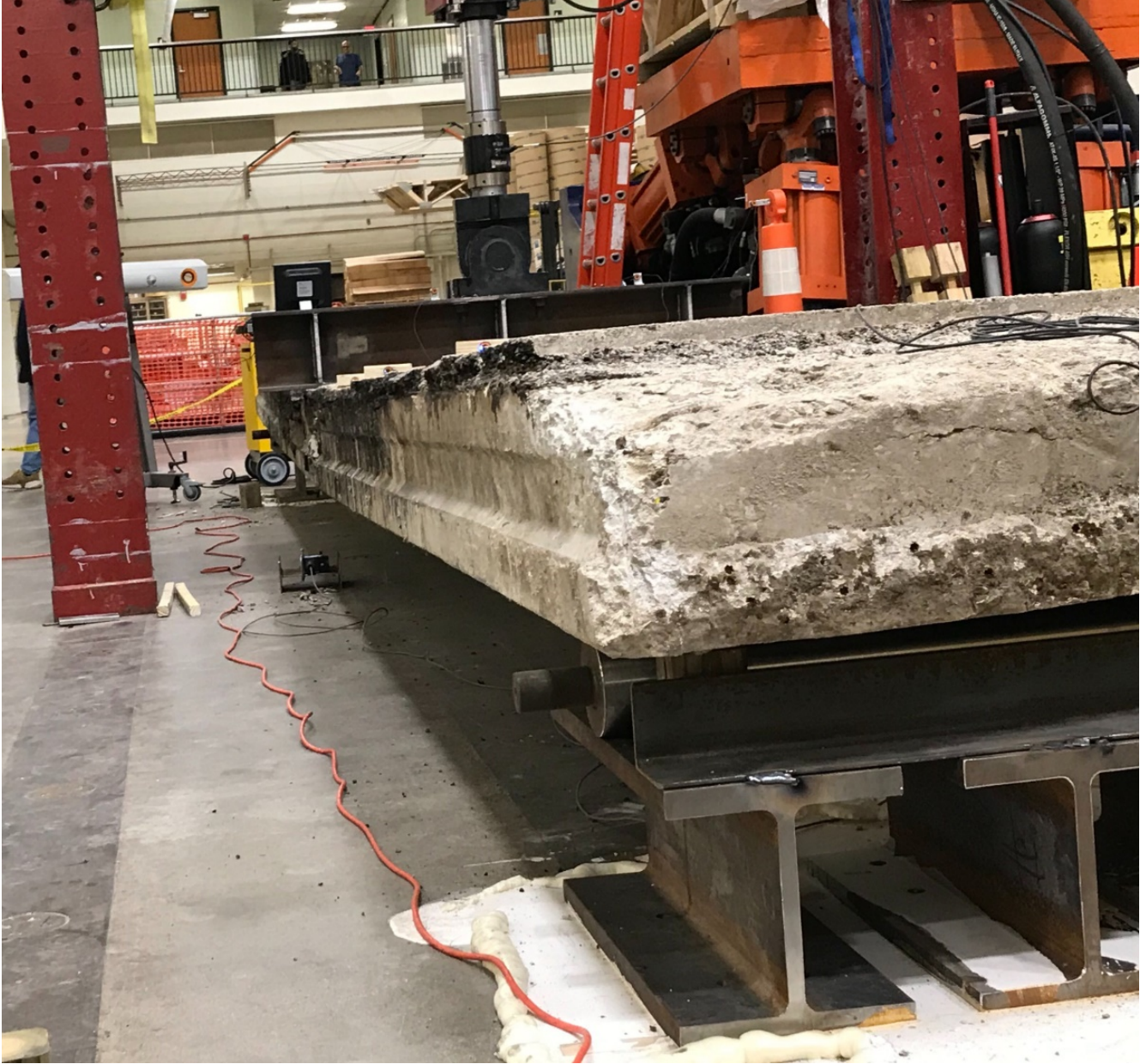
Figure 9. Photo. Test specimen during the three-point bending test.
